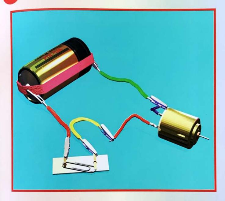
Push the paper clip against the brass paper fastener to close the loop and turn on the motor.
